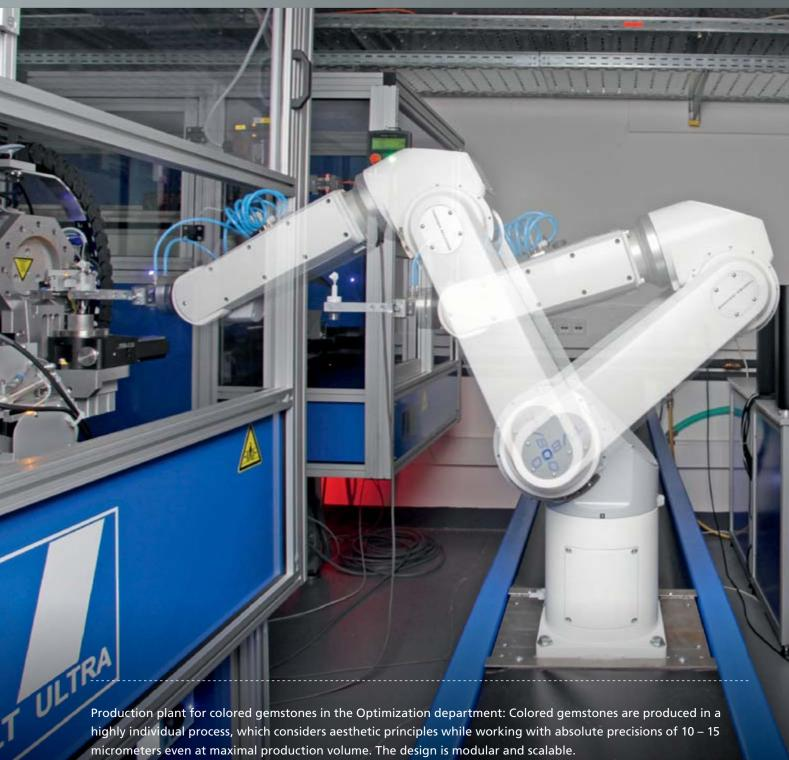
highly individual process, which considers aesthetic principles while working with absolute precisions of 10 – 15 micrometers even at maximal production volume. The design is modular and scalable.
