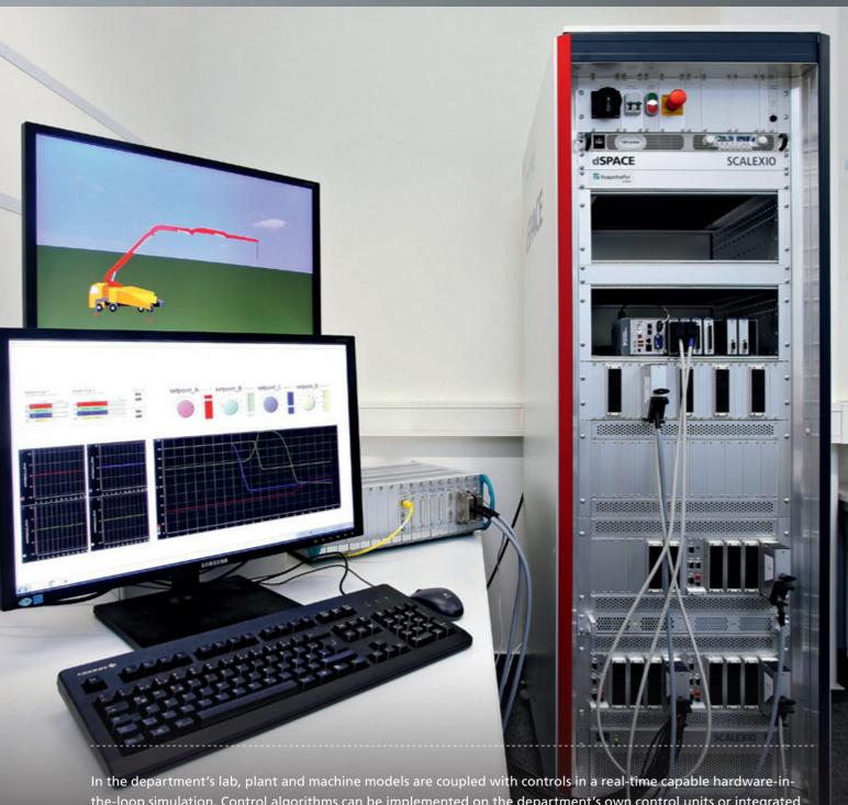
the-loop simulation. Control algorithms can be implemented on the department's own control units or integrated with the original client system. A comprehensively equipped HIL platform enables the data capture and generation of many different signal types in addition to error simulations.
