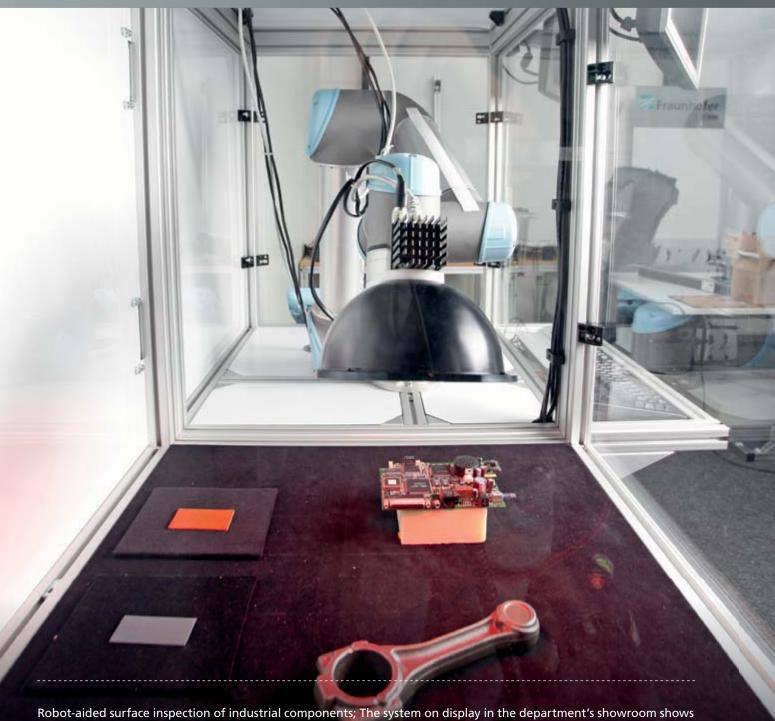
Robot-aided surface inspection of industrial components; The system on display in the department's showroom shows examples of two-dimensional and three-dimensional testing of different materials (leather, plastic, cast iron).
