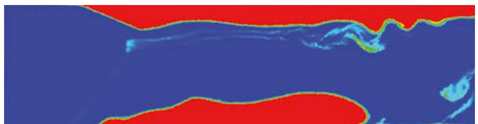
Mach3 step channel with turbulence model: turbulent kinetic energy
