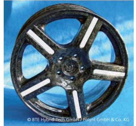
Fiber-reinforced polymers are applied as lightweight construction materials, for example for an especially lightweight rim.
