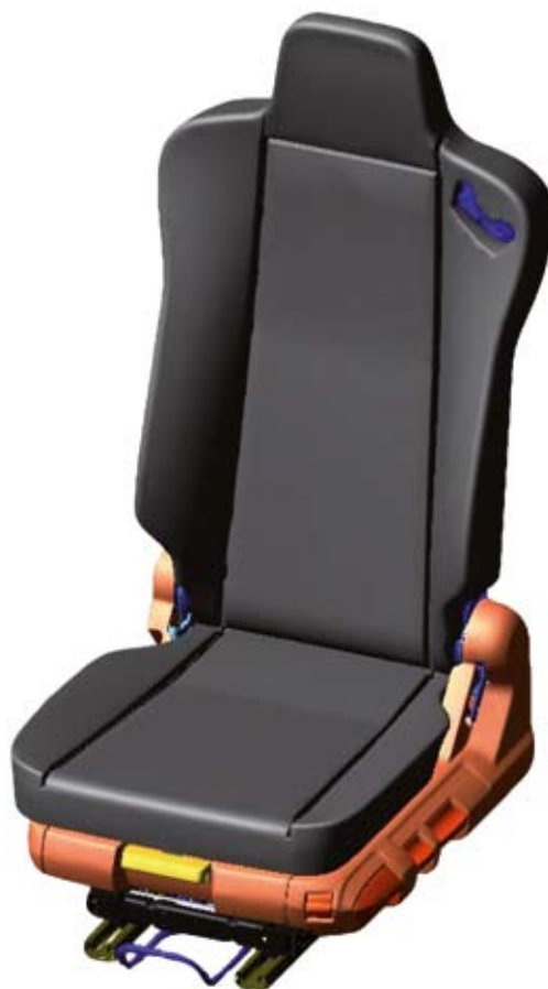
Virtual seat model for the simulation of the dynamic load, developed at the ITWM
