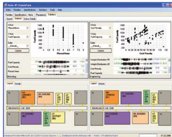
Decision support for the selection of configurations with maximum tank volumes: on the left, the reference configuration of the engineer, on the right, the configuration with maximum tank volumes
