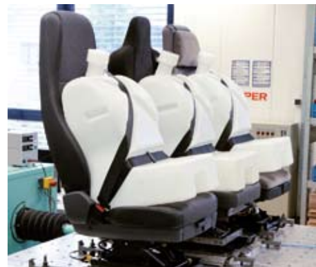
Test rig for the dynamic load to which seats are subject, at the company KEIPER
