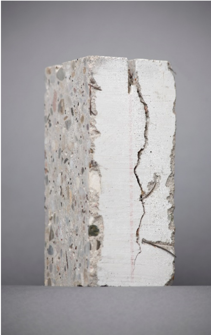
Picture 1 Concrete sample with crack.
